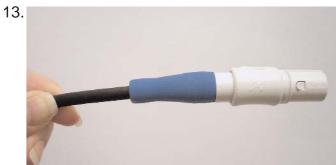
Strain relief installed
