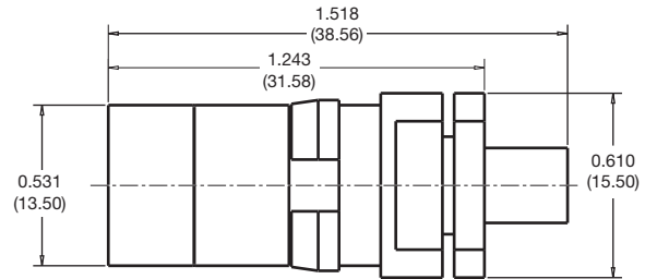
8.6 mm Crimp Socket for SFT142 Cable
