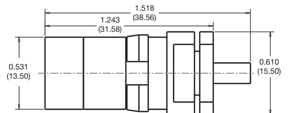
8.6 mm Crimp Socket for RG316 Cable
