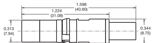
5.5 mm Crimp Socket for SFT142 Cable
